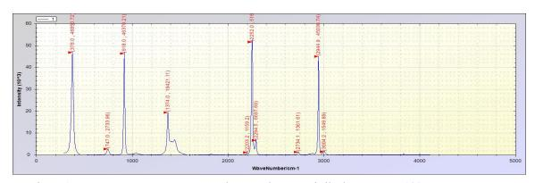
Figure 1 Raman spectrum curve test results; sample: acetonitrile, laser power: 130mW, measurement integration time: 4000ms.
